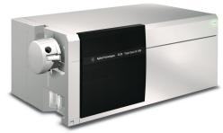
The Agilent 6420 Triple Quadrupole LC/MS delivers excellent sensitivity for routine analysis with performance specifications in Signal-to-Noise ratio (S/N) and Instrument Detection Limit (IDL). IDL is a rigorous, statistically based metric that indicates practical sensitivity performance of your quantitative assays. The 6420 Triple Quadrupole LC/MS achieves sensitivity and resolution specifications with autotune.
